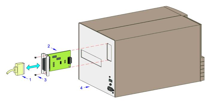
Figure 3-7, Interface Installation
